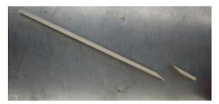
Now, from the opposing end that was just cut, mark 10" and cut a 45° angle. Regardless of whether you are making optional alterations to the neck or not, cutting approximately 10" off the end of the board is necessary. You will use this 10" section of wood to fasten the neck to the cardboard box. The optional portion of this step is the 45° angle. Set aside the 10" section of wood. At this point you are finished with the saw.
