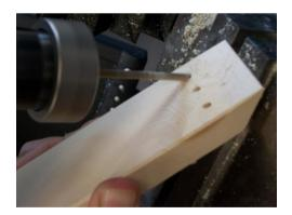
Now that the base of the neck finished you need to fasten it to the cardboard box aka the body of the guitar. Remember that 10" piece of wood you set aside; time to pull it back out. You will sandwich the box lid between the neck and the left over 10" board, refer to picture. Be careful to use the appropriate length screws, otherwise the screws tips will come through the front of your guitar's neck. You will use
