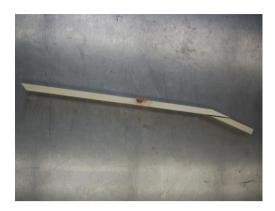
Next place the 15° angle cut piece on the underside of the longer piece and glue them together with wood glue. It is best if you clamp the pieces and allow them to dry for 24 hours before stressing them. The functional purpose behind having the neck at an angle is to create a downward force on the nut holding the strings which will help to maintain the correct tension in the string.
