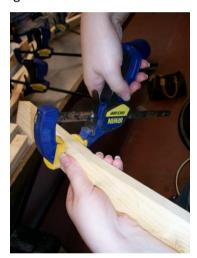
After the wood glue has dried completely, remove the clamp; you are now ready to sand down the joint made by gluing the two pieces together. Another optional aesthetic addition you can do with the sand paper is to sand a curvature about the end of the neck.
